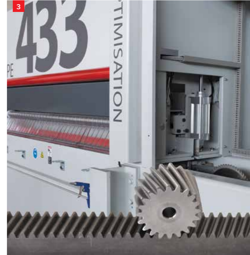
3 Araba Grubu Saw Carriage-Guidance System
