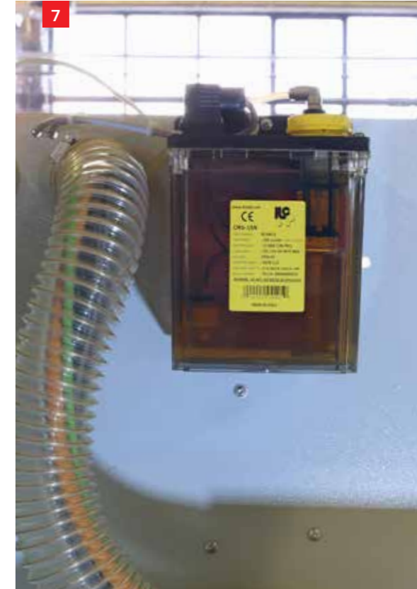
7 Otomatik Yağlama Sistemi Automatic Lubrication System
