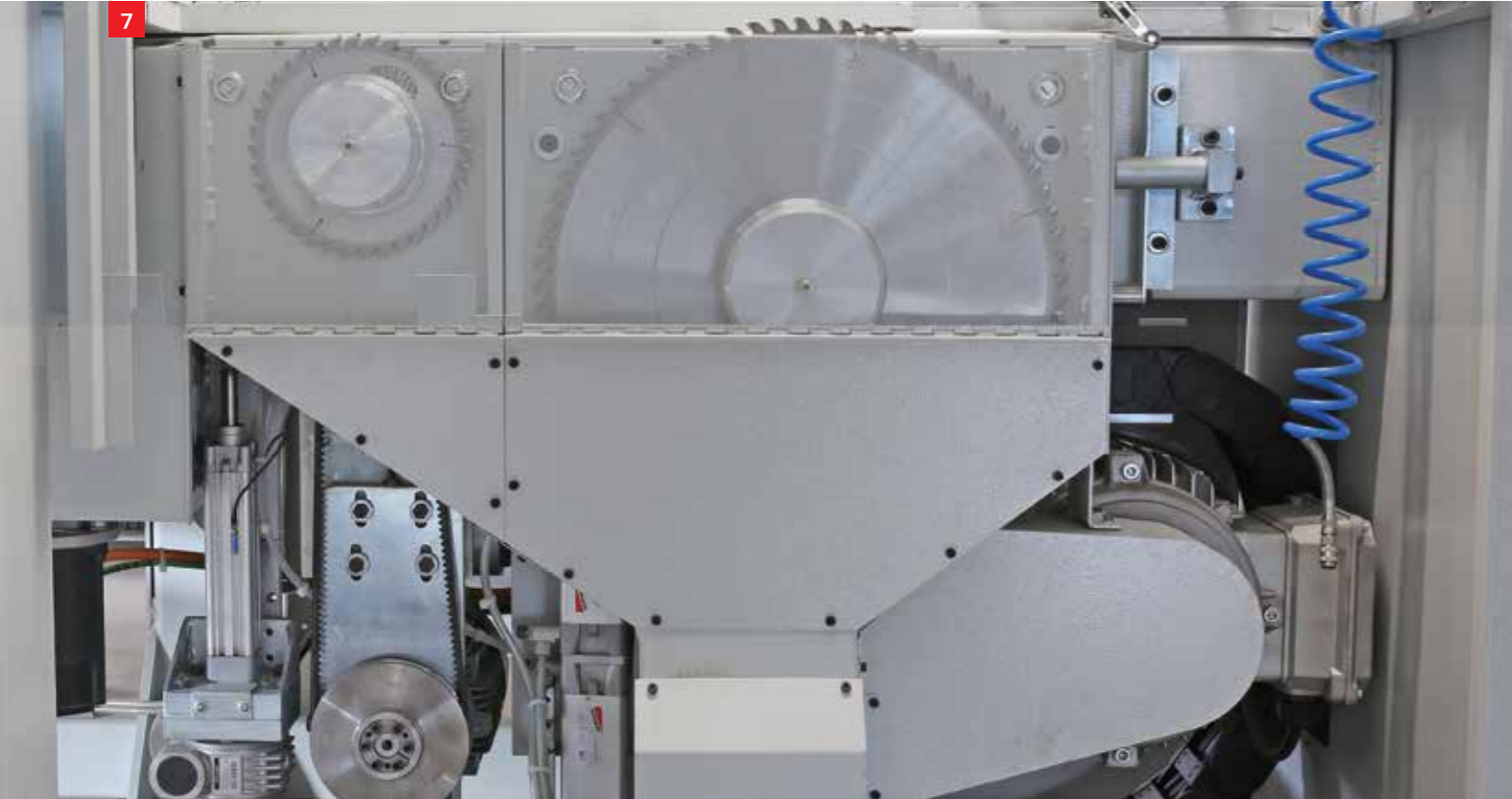
7 Araba Grubu Saw Carriage-Guidance System
