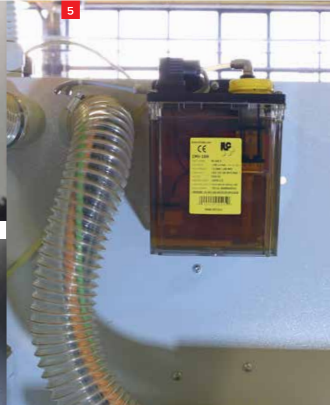
5 Otomatik Yağlama Sistemi Automatic Lubrication System
