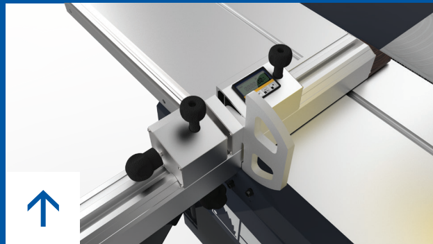
New crosscut fence stopper with precise adjustment system and electronic reader with absolute memory function and 0,1 mm accuracy (optional).
